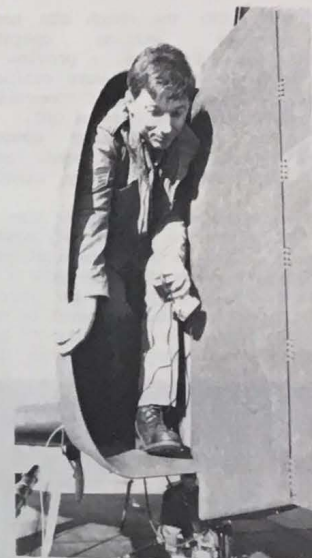
SSgt. Mike (Spike) Thompkins (Inspection Dock), exits an intake after checking the front of jet engine for any visible damage and foreign objects.
