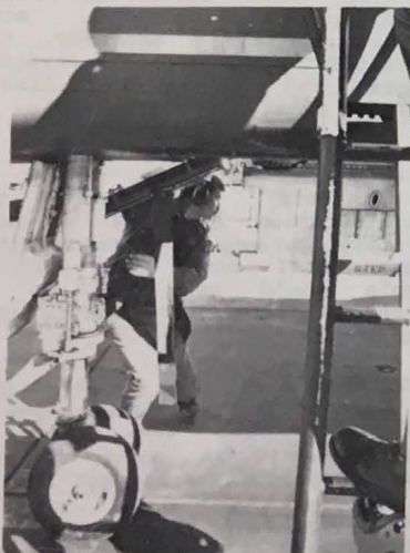
SrA. Brian Seaborn (fuel systems specialist) installs a landing gear down lock just after engine shut down.
